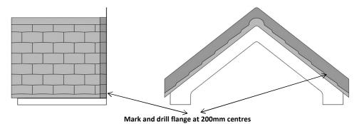
Mark out and pre-drill 6mm holes at approx 200mm centres along the canopy fixing flange (upstand).
